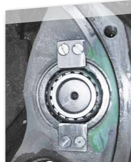
Repair of a gearbox casing Epoxy Resin Putty
