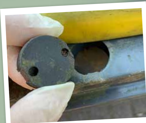
The plastic chip was cleaned with Cleaner Spray S before bonding.
