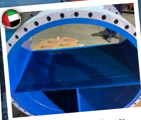
Coating of a heat exchanger
