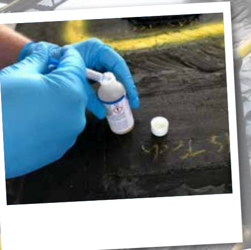
Then, WEICON Primer G was applied. The bonding agent ensures a better adhesive joint for surfaces that are difficult to bond - like rubber, in this case. That way, the adhesive bonding was ideally prepared. Then, the WEICON Urethane 85, which is included in the WEICON Belt Repair-Kit, was worked in and moulded to match the surface of the conveyor belt.
